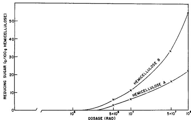
Figure 3. Sugar production from irradiated hemicellulose. Hemicellulose A and hemicellulose B (10% in aqueous solution) were irradiated at different doses, and the level of reducing sugar was determined by the DNS method.
