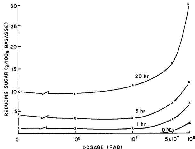
Figure 4. Effect of  $\gamma$  irradiation on enzymatic hydrolysis of sugarcane bagasse. The irradiated sample (0.25-g sample in 50 mL of 0.1 M acetate buffer, pH 4.5) was hydrolyzed with 50 mg of Onozuka cellulase at 50 °C.
