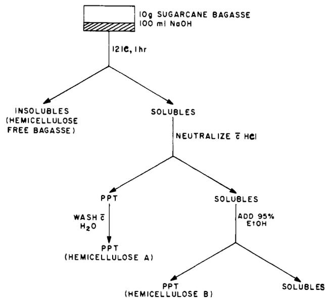
Figure 1. Isolation scheme for hemicellulose from sugarcane bagasse.
